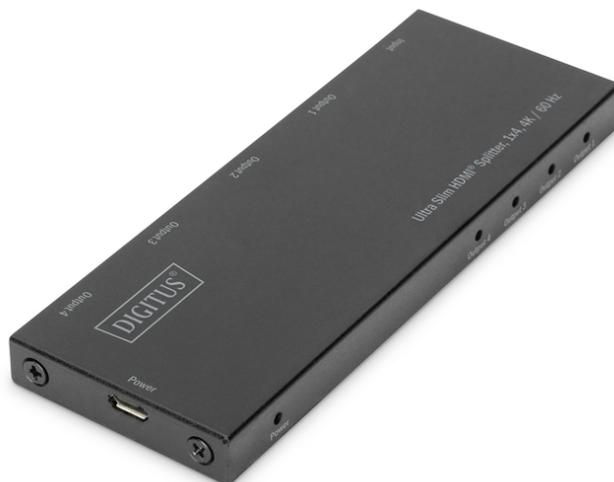
**Ultra Slim HDMI Splitter, 1x4, 4K/60Hz HDR, HDCP 2.2, 18 Gbps, Micro USB Power**
